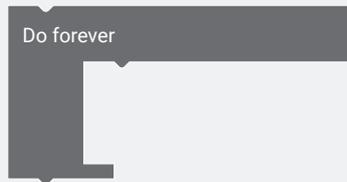
This block is an endless loop. Inserted blocks are called again and again. However, the Oxocard has an «auto-turnoff» function. This automatically switches off the Oxocard after 2 minutes of inactivity.
